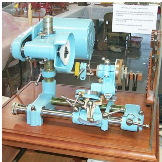
[Editor] I was not sure what a Quorn Tool and Cutter Grinder looked like and found this lovely example online.
